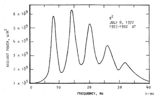
Figure 4. High-Resolution Measurement of Schuman-Wave Radiation Near Kingston, RI
