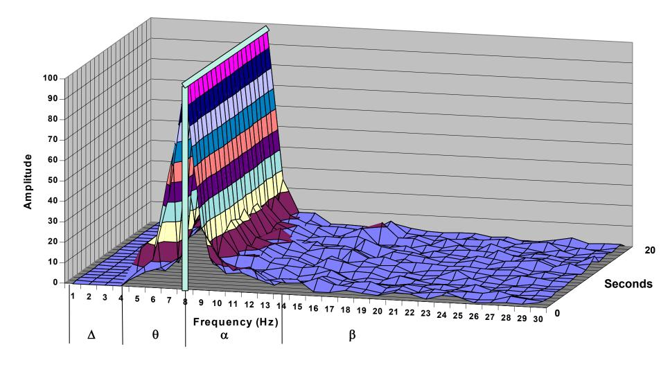
Figure 6. FFT of complete system with 7.81 Hz input signal
