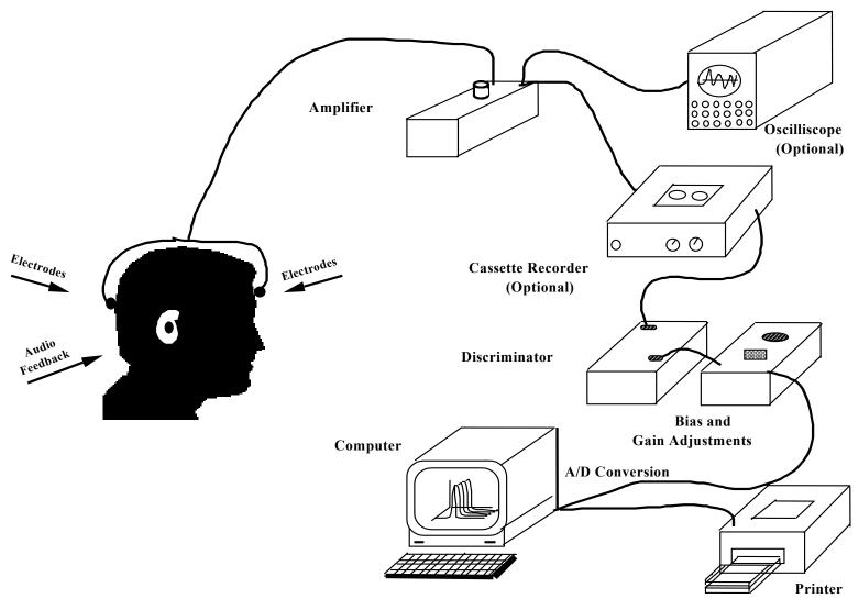
Figure 7. EEG frequency display system
