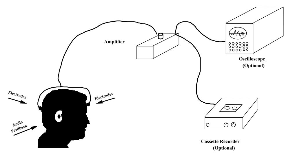
Figure 5. Beck's EEG biofeedback system
